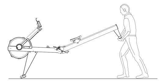
4. The MAIN FRAME(1) and the RAIL FRAME(2) can be separated to minimize the unit size for storage. Remove the PULL PIN(98) from the MAIN FRAME(1). Lift up the MAIN FRAME(1) and pull out the RAIL FRAME(2) to separate. Insert the PULL PIN(98) back to the hole in the MAIN FRAME(1) for storage.
